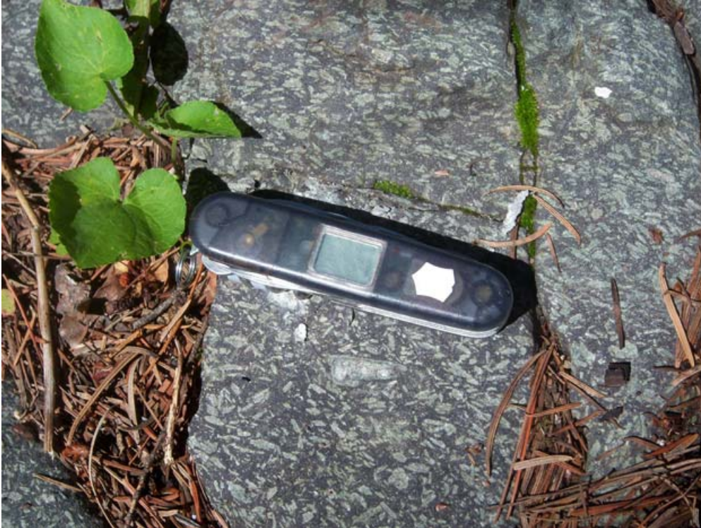
Figure 11: Example of “turkey track” basaltic trachyandesite (Twtx) exposed at confluence of Argentina and Little Argentina Creeks. Plagioclase phenocrysts may be two or three times larger in some flows.
