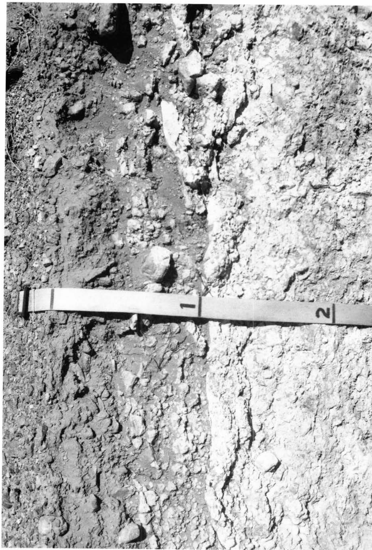
FIGURE 12—Upper horizons of the Typic Petrocalcic, Delnorte 67-2, in Jornada I alluvium at study area 23c. Platy, light-colored fragments above the continuous surface of the Km horizon (at 1 ft depth) once were part of continuously cemented laminar horizons. The fragments occur just above the Km horizon (particularly at the right) and extend upward about half way to the soil surface. Scale is in feet. Photographed June 1967.
