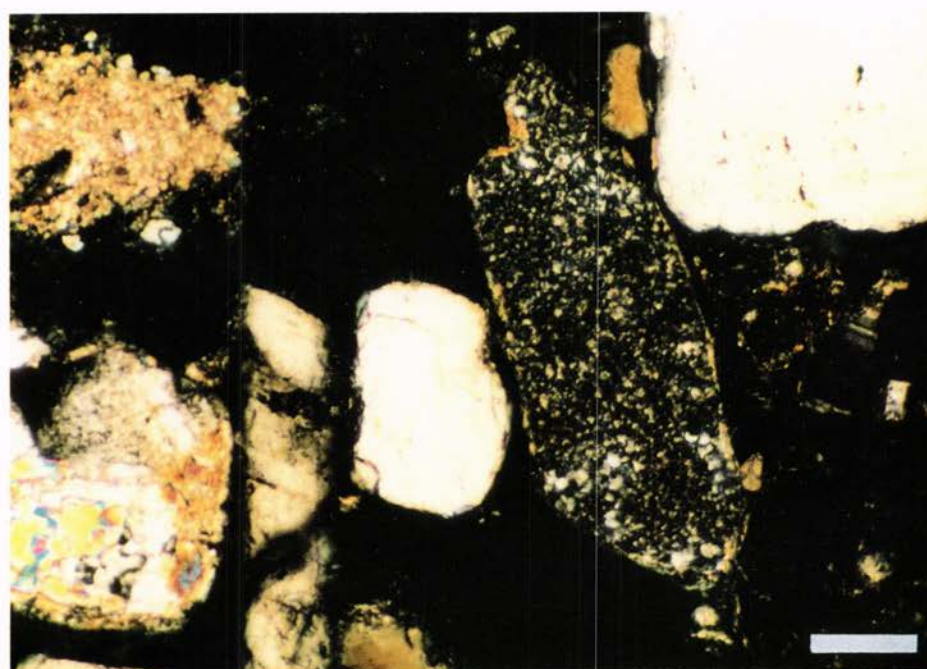
PLATE 23—Thin section of the C1 horizon of the Typic Petroargid, Rotura, at study area 26. Arrows locate opal miniscus bridges between grains, which are mostly quartz and rhyolite. Upper, plane-polarized light; lower, crossed polarizers. Bar scale = 100 \mu\text{m} .
