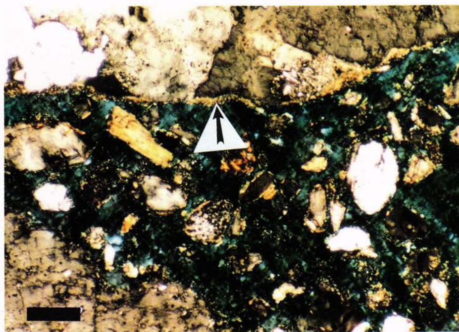
PLATE 11—Thin section of the Ck horizon of the Typic Haplocambid, Pajarito, at study area 10a. Thin stage I carbonate coatings (grain calcitans) occur on many grains; arrow locates a thin calcitan on the large grain at top. Monzonite is dominant, with some feldspar, quartz, and a minor amount of biotite. Upper, plane-polarized light; lower, crossed polarizers. Bar scale = 100 \mu m.
