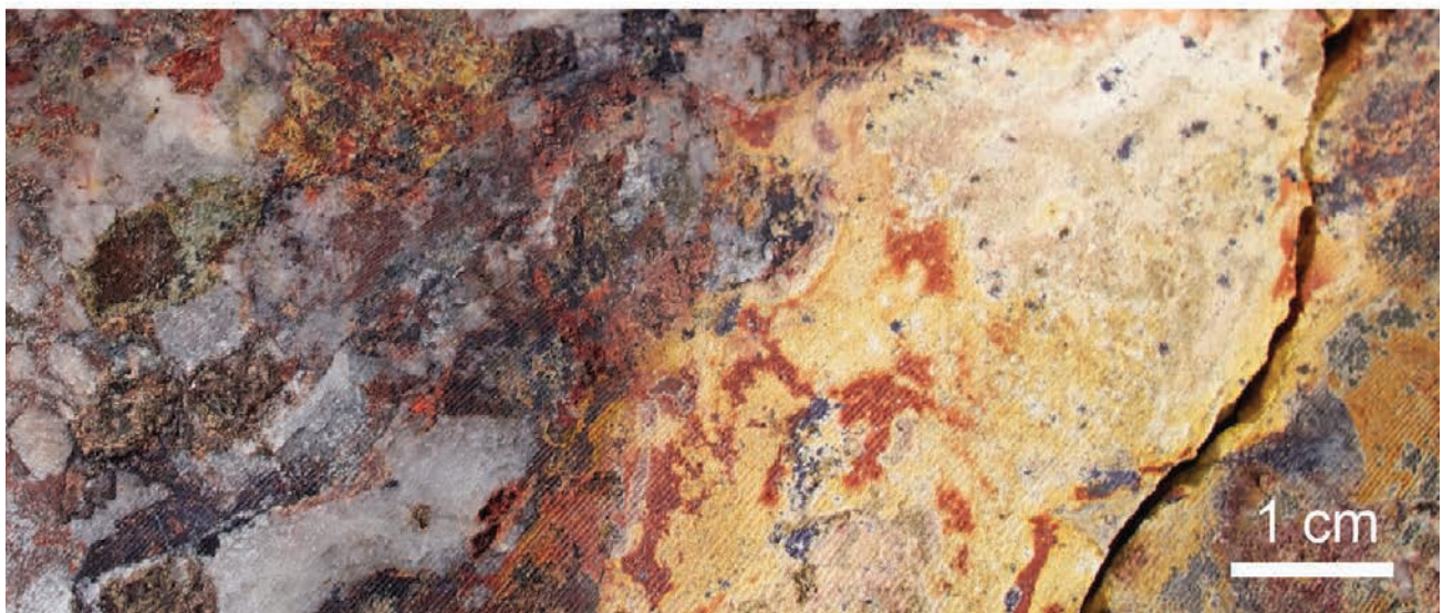
Rock scans of mineralized pegmatites overprinted by hydrothermal alteration from the Strange Lake REE-Zr-Nb deposit, Quebec, Canada. Photo by A. Gysi
