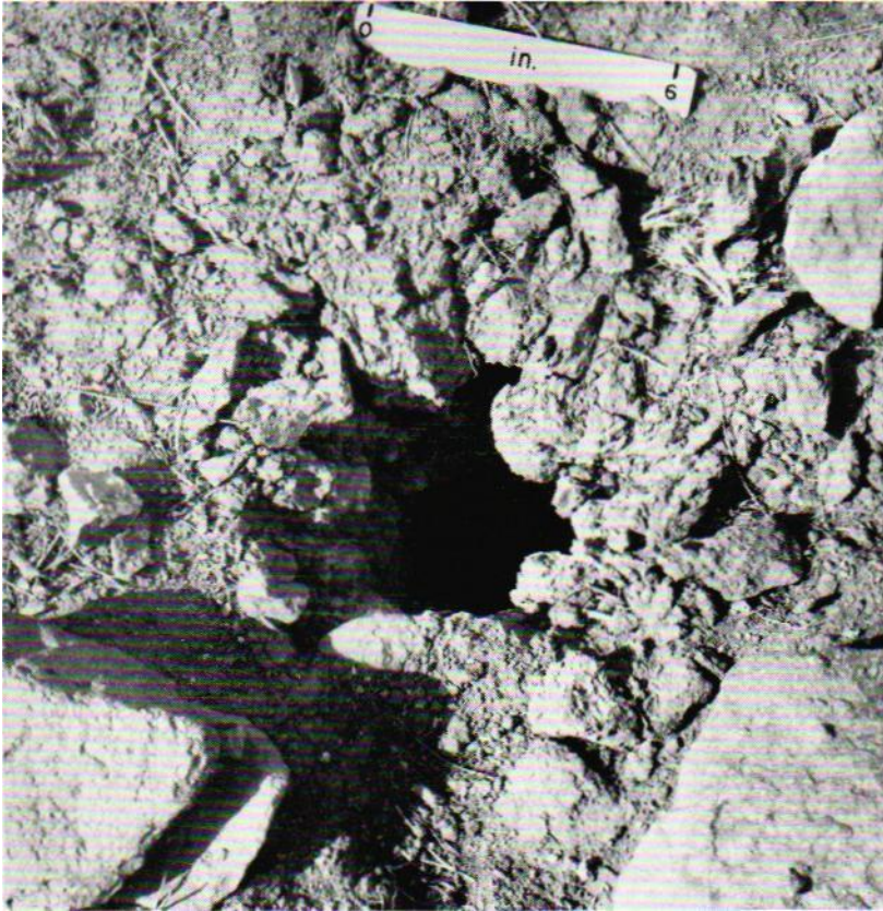
Figure 9 CRATERLESS HOLE SHOT INTO ALLUVIUM WITH A 4-INCH- DIAMETER CAST IRON LINER
