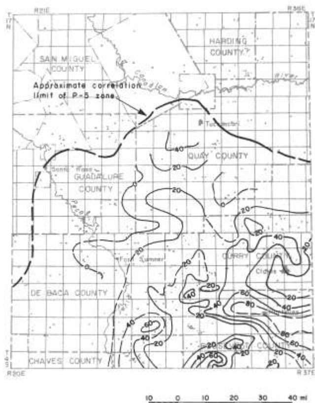
FIGURE 17—THICKNESS IN FEET OF P-5 ZONE WITH 10+ PERCENT POROSITY; contour interval equals 20 ft.
