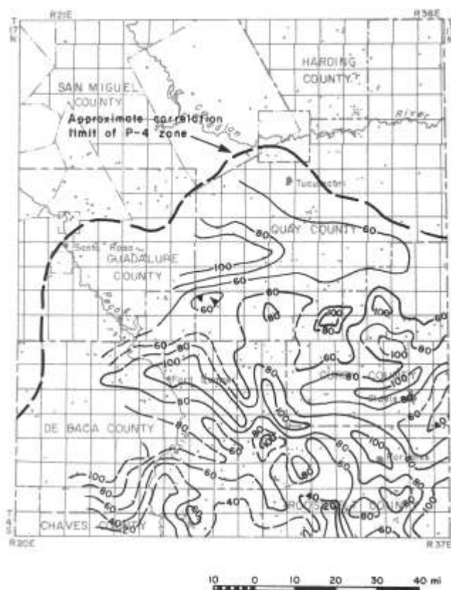
FIGURE 12—PERCENT OF DOLOMITE IN P-4 ZONE; contour interval equals 20 percent.
