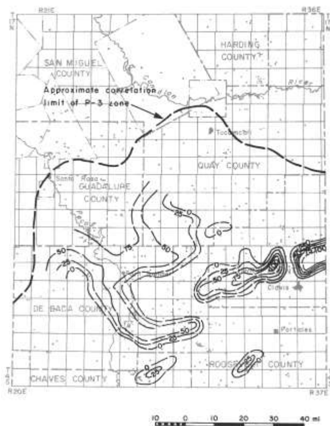
FIGURE 10—PERCENT OF SALT WITHIN EVAPORITES OF P-3 ZONE; contour interval equals 25 percent.
