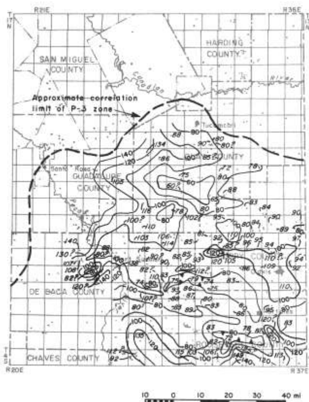
FIGURE 6—ISOPACH MAP OF P-3 ZONE; contour interval equals 20 ft, depths of well measurements shown in feet.
