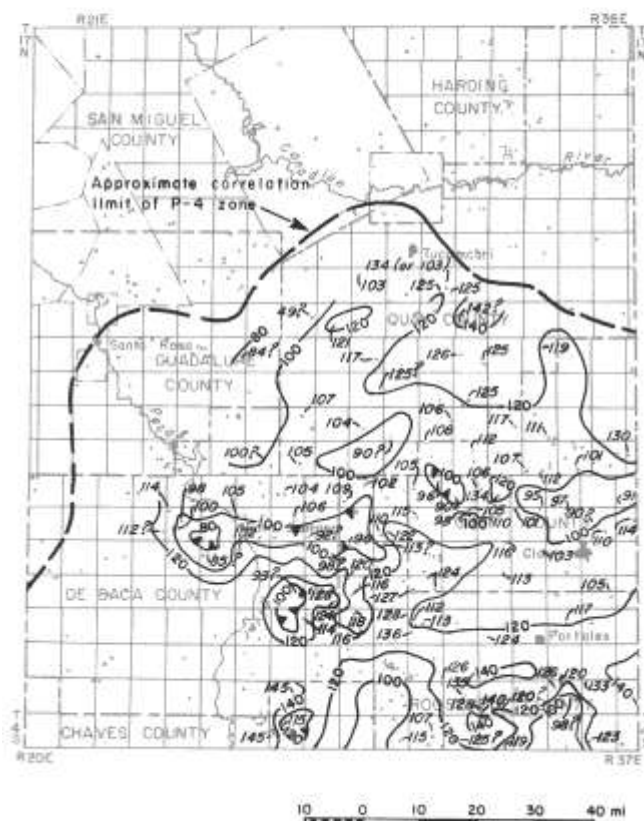
FIGURE 11—ISOPACH MAP OF P-4 ZONE; contour interval equals 20 ft, depths of well measurements shown in feet.
