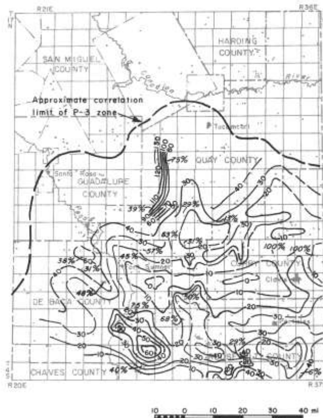
FIGURE 9—EVAPORITE THICKNESS OF P-3 ZONE; contour interval equals 10 ft, percent of salt present shown by %.
