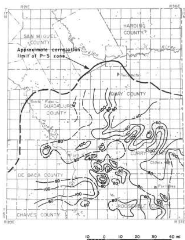
FIGURE 16—PERCENT OF DOLOMITE IN P-5 ZONE; contour interval equals 20 percent.
