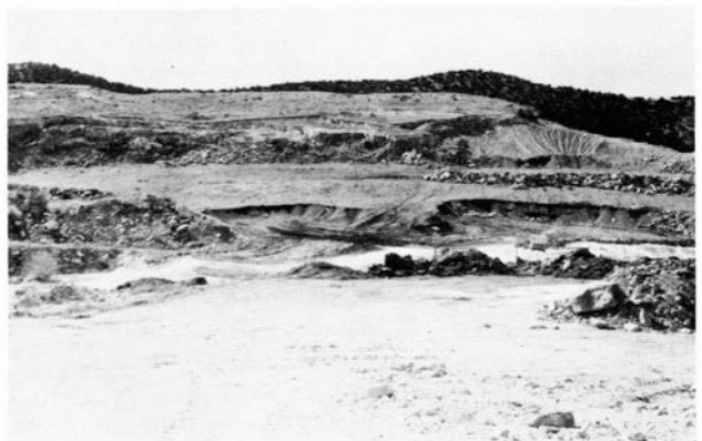
FIGURE 79—QUARRY OF IDEAL CEMENT CO. WEST OF PLANT. LIME KILN BED WHICH HAS PRINCIPAL LIMESTONE SOURCE IS IN FACE OF SHALLOW QUARRY. "RED BED" SHALE ALSO QUARRIED IN LOWER SHALLOW CUT, IS JUST BELOW THE LIMESTONE.
