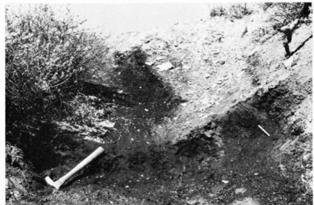
FIGURE 85—COAL OUTCROP AT LEFT SIDE OF PINA VITITOS MINE PORTAL. BOTTOM OF SEAM AT HAMMER HEAD; TOP, AT PENCIL.
