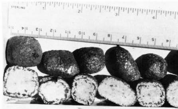
E—ORBICULE CORES; CENTER-SAWED. NOTE RECTANGULAR SHAPE AND FIRST BIOTITE WRAP; SECOND WRAP AROUND COARSE FELDSPAR CORE IS SHOWN ON HALVES LYING FACE-DOWN.
