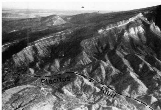
FIGURE 61—AIRVIEW TO THE SOUTHEAST SHOWING NORTHERN END OF SANDIA MOUNTAINS. UPPER RIGHT SHOWS BRUSH-COVERED SLOPE ERODED ON SANDIA FORMATION OVERLYING CLIFFS OF SANDIA GRANITE. STRONGLY LEDGED CREST AND EAST DIP SLOPE IS MADERA FORMATION. CENTER AND LOWER RIGHT SHARP, ERODED HOGBACK HILLS ARE CAPPED BY NORTH-DIPPING MADERA BEDS FAULTED DOWN AND ROTATED TO FORM THE NORTH RAMP TERMINATION OF THE UPLIFT. ON THE UPLIFT BACK SLOPE CAN BE SEEN PALOMAS PEAK AND OTHER SMALL PIGGYBACK FAULT BLOCKS.
