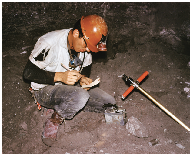
Figure 7. Geologist measuring the grade of ore in Section 25 mine (NMMK0220), Ambrosia Lake subdistrict during the 1970s. Photo provided by William L. Chenoweth, from the U.S. Atomic Energy Commission Historical Photo Collection.
