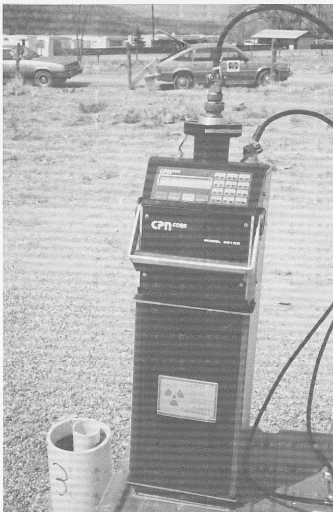
PHOTOGRAPH 6—Equipment used for monitoring in situ moisture and density conditions.
