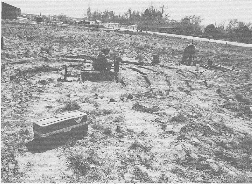
PHOTOGRAPH 7—Geotechnical ground stabilization study area 3 (GGSS-3) showing surface settlement and ground cracks (view to the south).
