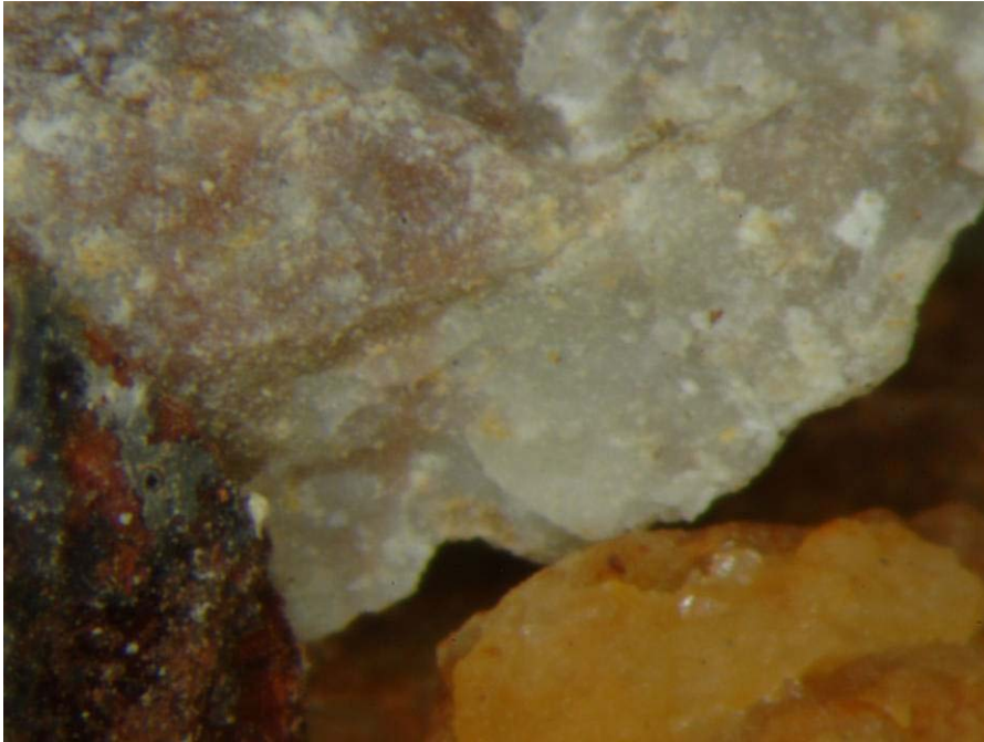
FIGURE 1-20. Sample QPS-AAF-0005 showing Amalia Tuff grains with Fe-oxide coatings (field of view is 6mm).
