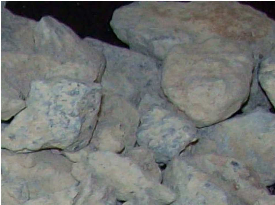
FIGURE 1-14. Sample MIN-SAN-0002 with subrounded shape of clast with some F-oxide stains (field of view is 4mm).
