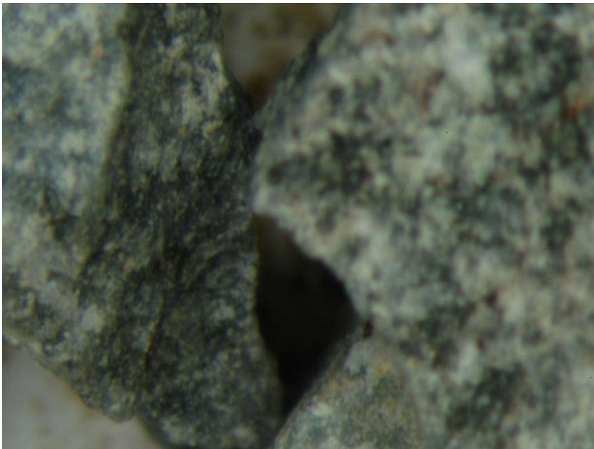
FIGURE 1-26. Sample SPR-SAN-0002 with QSP and propylitic alteration on andesite rock fragments (field of view is 6mm).
