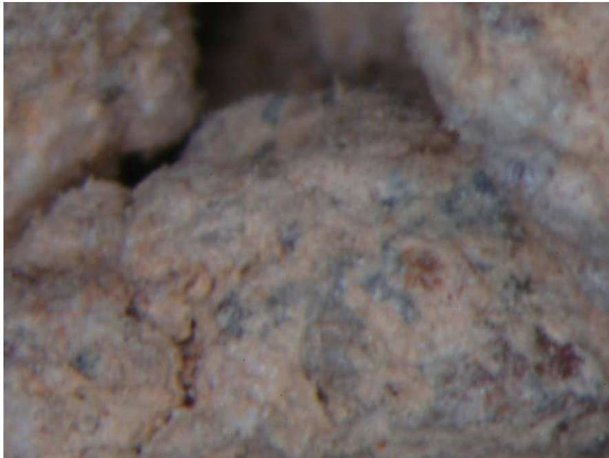
FIGURE 1-24. Sample QPS-SAN-0002 with andesite and intrusive rock fragments with iron coatings (field of view is 6mm).
