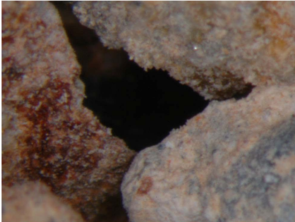
FIGURE 1-18. Sample QPS-AAF-0003 with gypsum as cementing mineral. Iron coating on rock fragments (field of view is 6mm).
