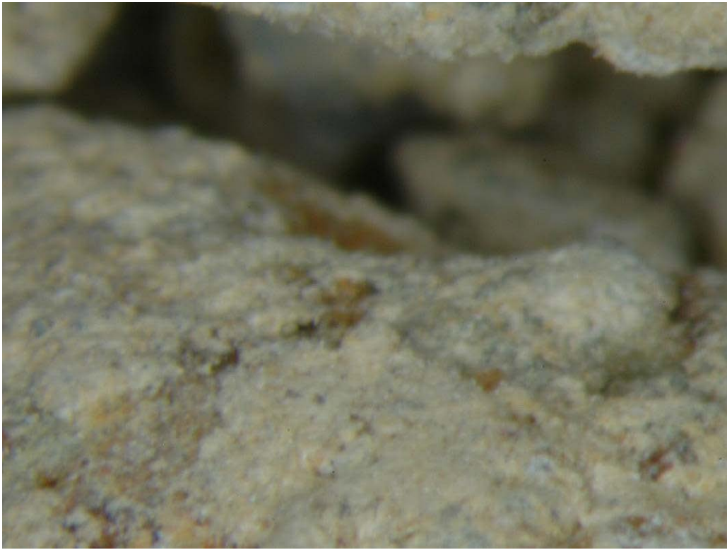
FIGURE 1-22. Sample QPS-AAF-0009 with Amalia Tuff rock fragments with few iron coatings (field of view is 6mm).
