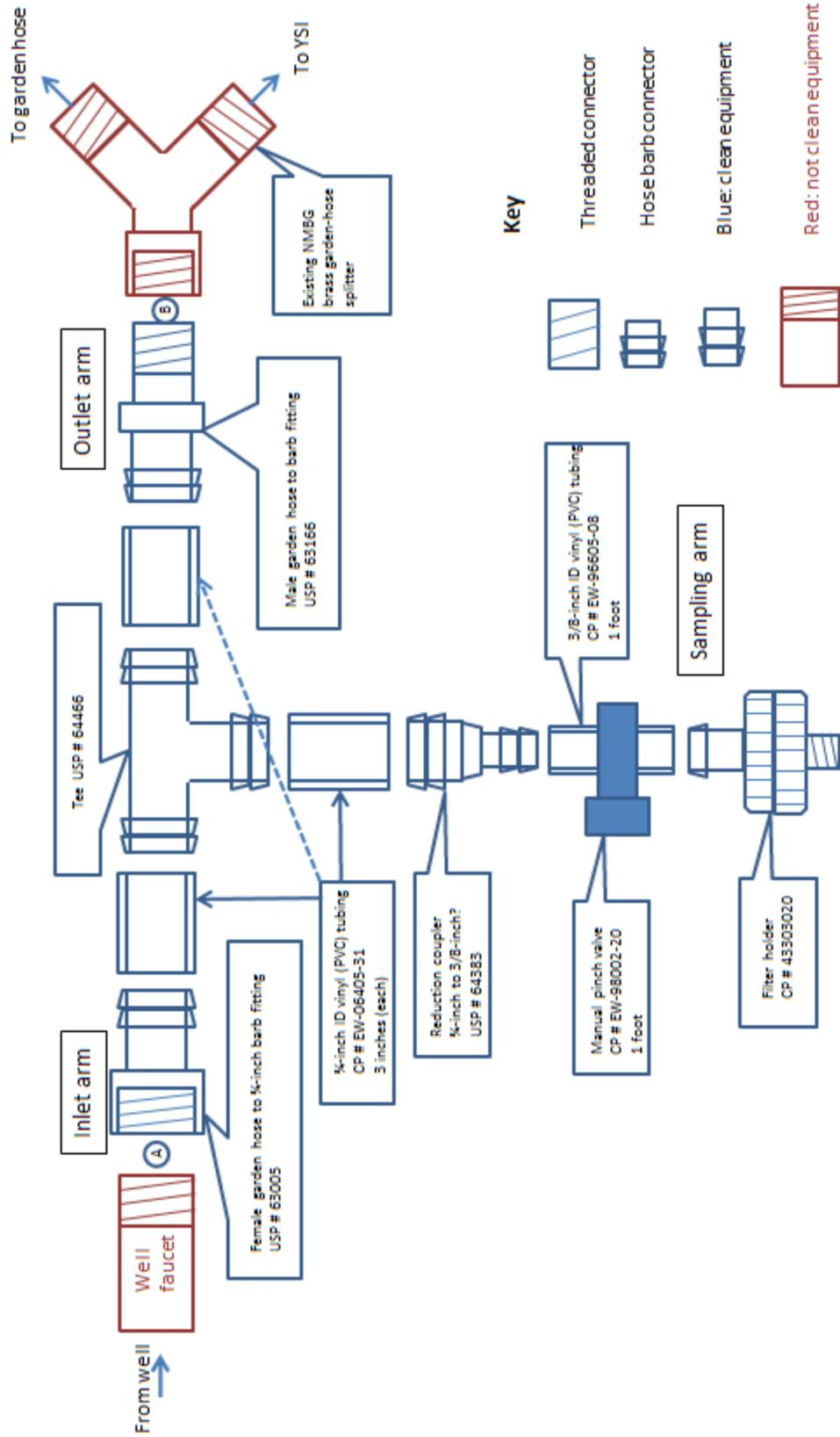
Figure 1. Sampling manifold and filter holder
