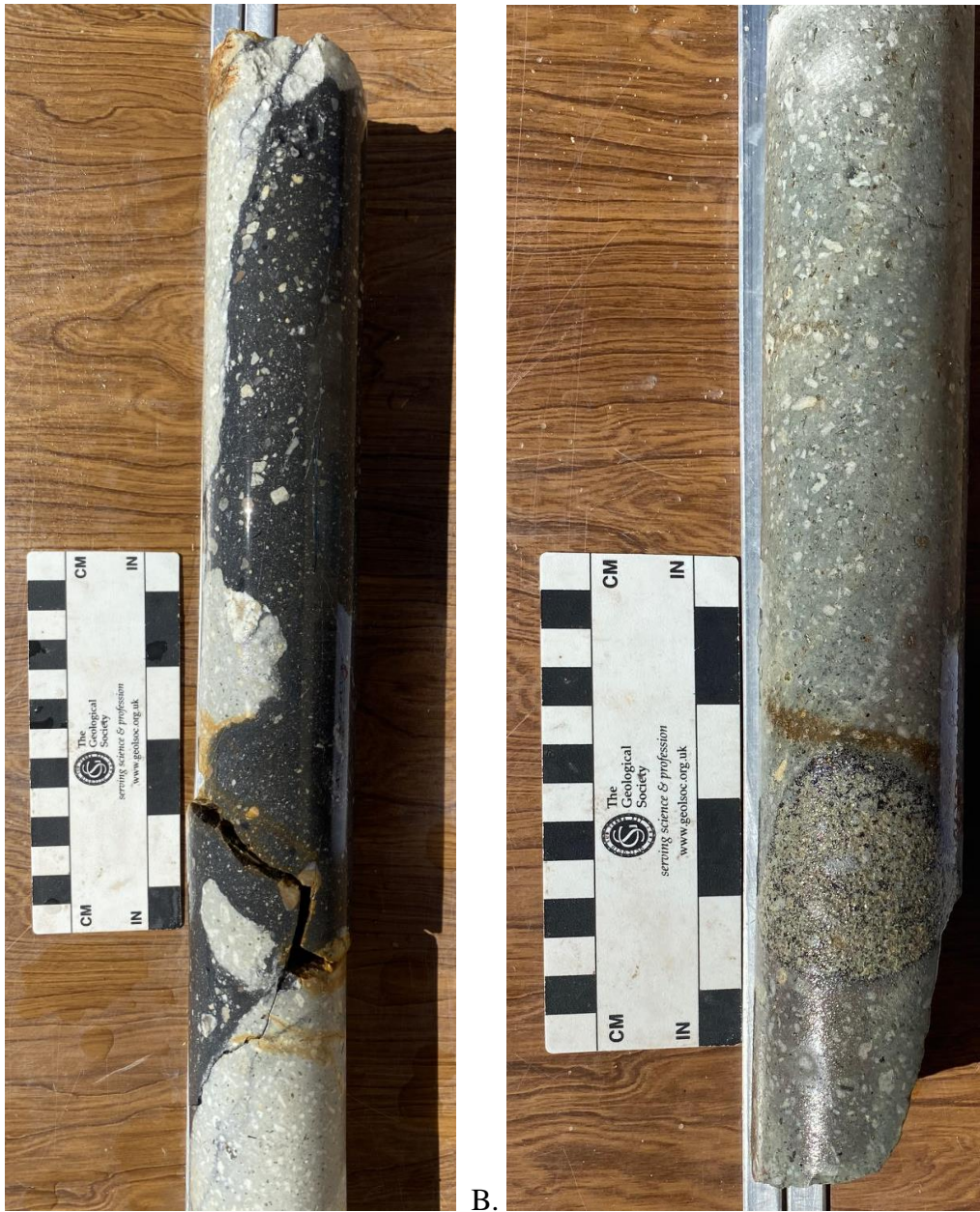
FIGURE 52. A) Breccia dike (black) cutting syenite dike, Chess Draw, Hole C-1, 217.5 ft depth. B) Breccia dike (black) cutting syenite dike, Chess Draw, Hole C-1, 139.2 ft depth. Note the round nepheline syenite rock fragment at the bottom of the core.
