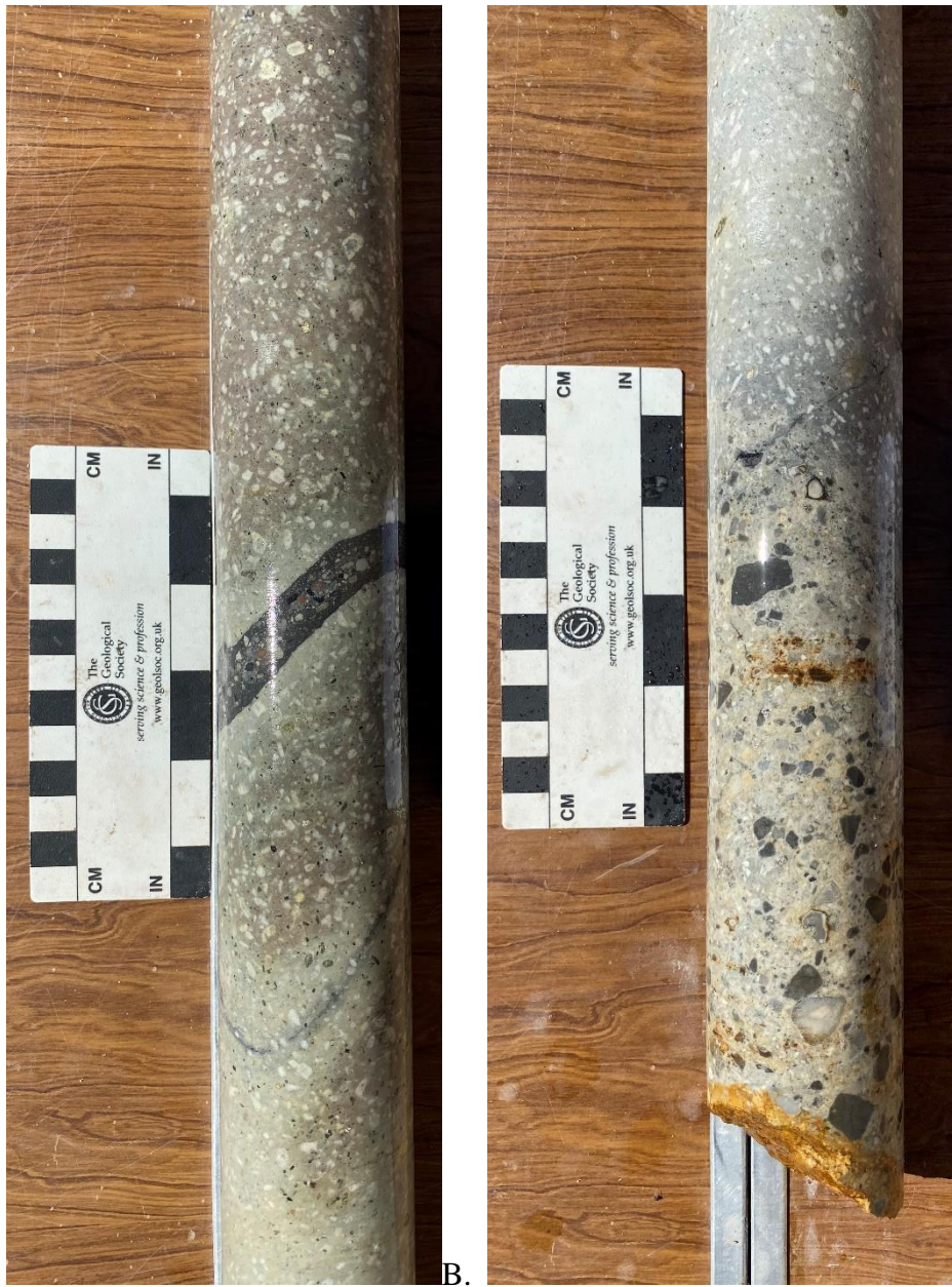
FIGURE 53. A) Thin black breccia dike intruding trachyte dike, Chess Draw (drill hole C-1, 177.0 ft depth). B) Volcanic breccia (Chess Draw Hole C1, depth 224.0 ft). Dark fragments are phonolite; light gray fragments are trachyte.
