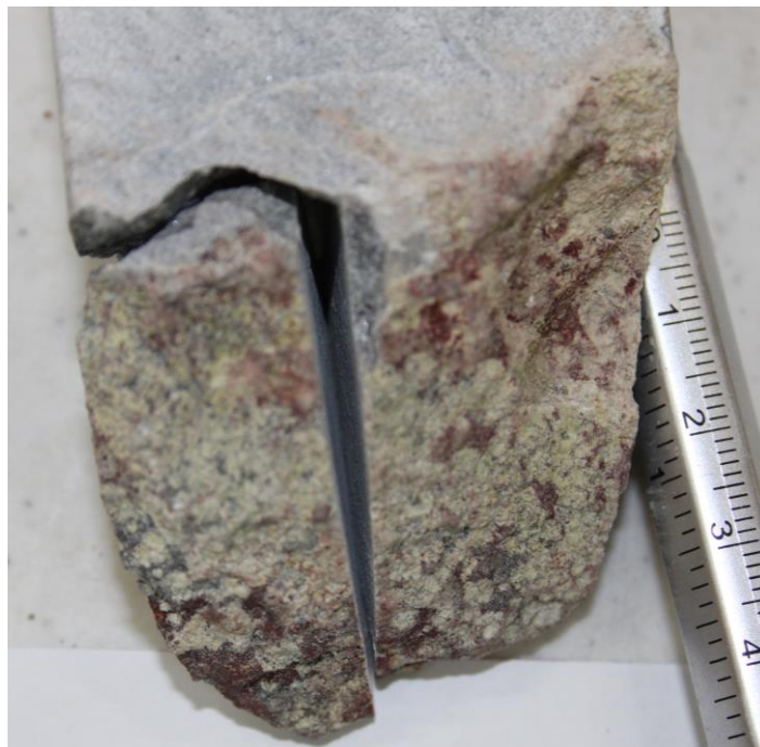
FIGURE 119. Eudialyte in nepheline syenite, 1473.35 ppm total REE, 8826 ppm Zr (WMEB-2, 541.5 ft).
