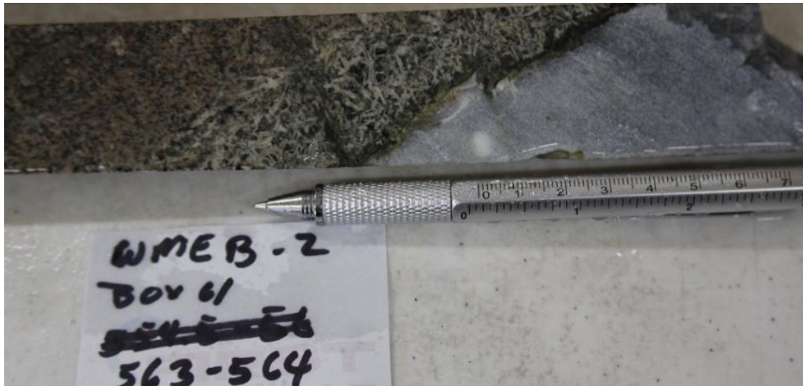
FIGURE 43. Nepheline syenite intruding unaltered limestone (Wind Mountain core, WMEB-2, depth 563-564 ft). Note thin layer of skarn at contact.
