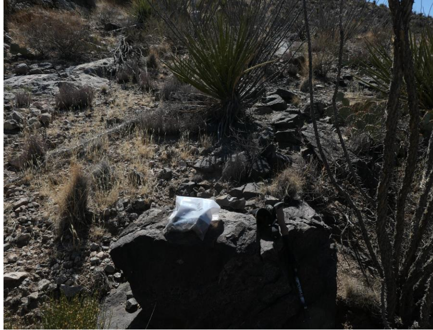
FIGURE 105. Phonolite dike intruding Hueco limestone near the contact with the skarn. Samples of phonolite contained 3513.08 ppm total REE (CORN242). Note limestone outcrops in upper left of photograph.
