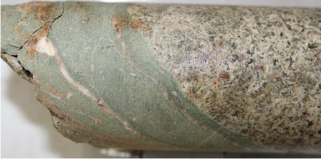
FIGURE 44. Contact between nepheline syenite and green skarn or tactite (metasomatized shale or siltstone; Wind Mountain core, WMEB-4, depth 229.1-229.7 ft).
