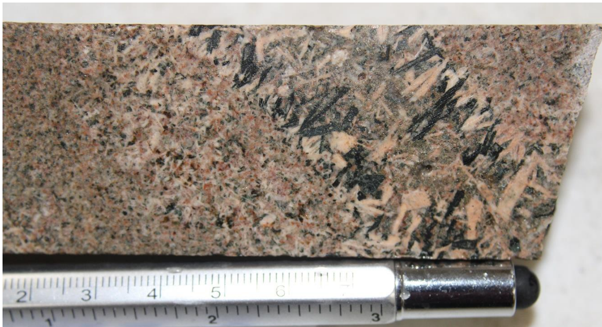
FIGURE 14. Amphibole-rich pegmatite cutting nepheline syenite (PEnsp2, drill hole WMEB-4, depth 400 ft, total REE=703.86 ppm, 2991 ppm Zr).
