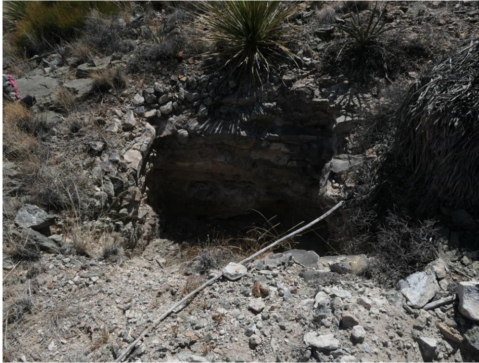
FIGURE 103. Skarn in Hueco limestone near phonolite dike (NMOt043). Pit is approximately 4 ft deep. Composite sample across the skarn (3 ft) contained 1599.55 ppm total REE (CORN239).
