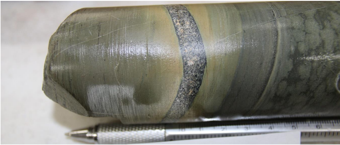
FIGURE 49. Nepheline syenite dike intruding a skarn or tactite (WMEB-6, 127.5 ft).
