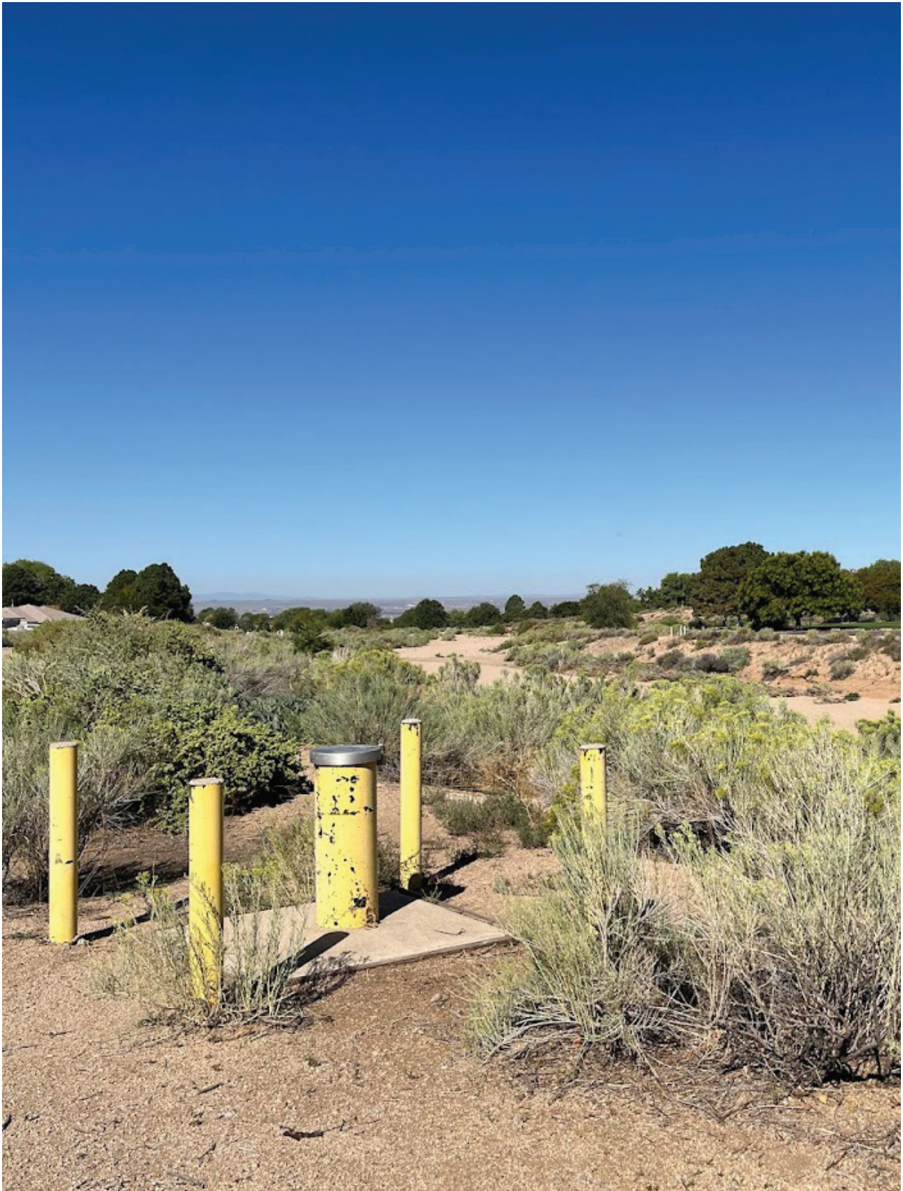
A groundwater monitoring well at the ABCWUA Bear Canyon Recharge Project. Photo by Rowan Hannan, ABCWUA
