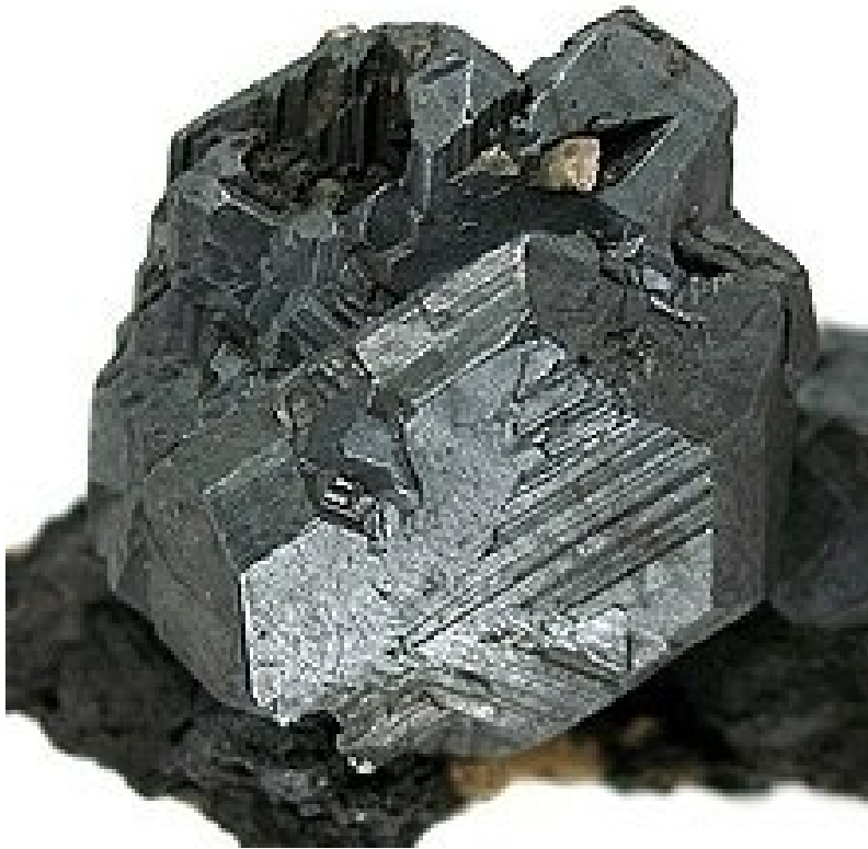
Chalcopyrite – Copper Sulfide Processed by FLOTATION
