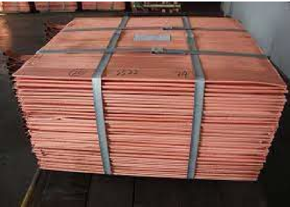
Copper Cathodes Processed after LEACHING
