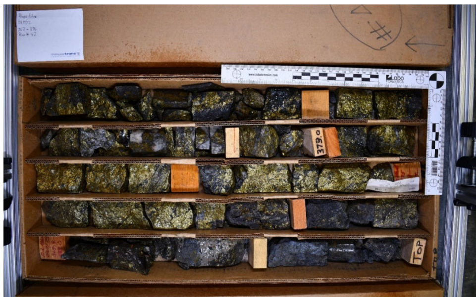
FIGURE 24. Mineralized skarn deposits showing chalcopyrite and magnetite mineralized zones in drill core from the Pinos Altos district, hole PAPD2, interval (ft) 367–376, box 42 (K. Stafford photograph).
