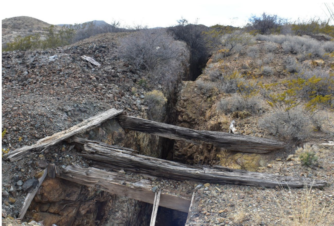
FIGURE 48. Open stopes along a skarn in the American mine, Eureka district, Little Hatchet Mountains (V.T. McLemore photograph, looking southeast).
