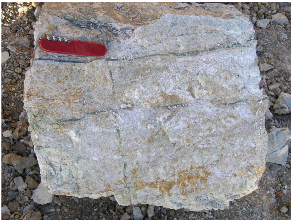
FIGURE 36. Typical gray porphyry copper-molybdenum veinlets at Chino, Santa Rita district (V.T. McLemore photograph).
