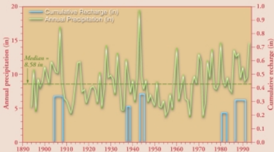
Figure 2. Annual precipitation and simulated ground-water recharge, Jornada Research Facility, Doña Ana County, New Mexico 1892–1991 (Kearns and Hendrickx, 1998). Reference line reflects median precipitation.
