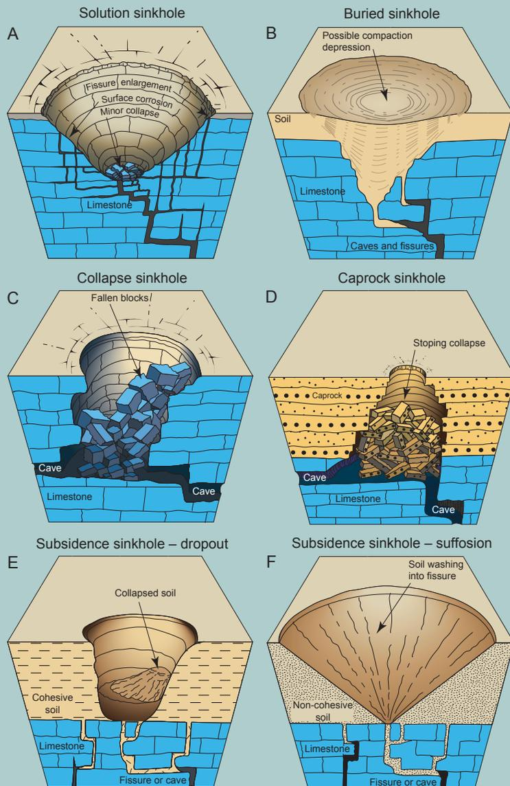
*Mechanisms of sinkhole formation. Modified from Waltham, 2008, Quarterly Journal of Engineering Geology and Hydrogeology, v.41, p. 292.*
