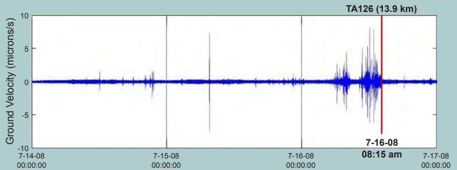
A July 2008 three-day seismograph record of vertical ground velocity measured by seismometer TA126, located approximately 13 km (8 mi) from the JWS brine well, showing more than six hours of ground motion leading up to sinkhole formation. The estimated time of surface breaching (8:15 am) is depicted by a vertical red line. By Lewis Land.
