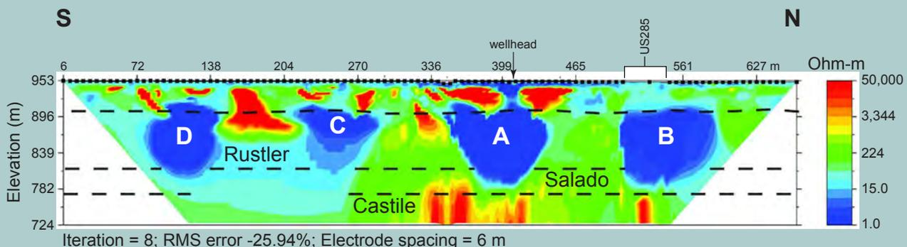
Profile of ER array line INW4 showing four distinct cavities in blue (A–D); black dots show individual electrode locations. The names Rustler, Salado, and Castile indicate the geologic formations represented in the cross section. By Lewis Land.
