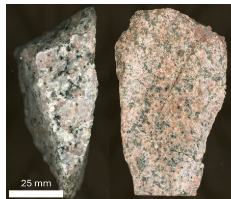
Color variation in scanned and polished samples of Sandia granite. In these hand samples, you can see the four main minerals that make up the Sandia granite. The pink mineral is microcline, the white mineral is plagioclase, the clear or gray mineral is quartz, and the black minerals are mostly biotite. The color and texture vary greatly across the pluton. Images by Nels Iverson
