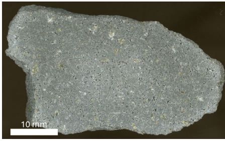
A polished slab of Carrizozo lava, showing a gray color and fine-grained texture. Most of the gray is composed of very fine-grained plagioclase feldspar and pyroxene. The green minerals are olivine. Dark spots are void spaces called vesicles. Image by Nels Iverson
