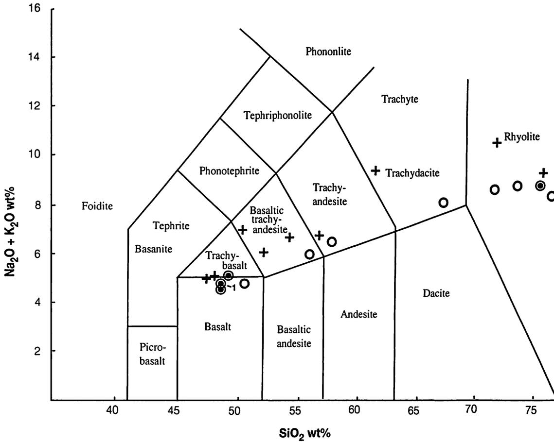
**FIGURE 2. Diagram of weight percent total alkalis versus silica for volcanic rocks in the Last Chance and Saline Ranges. ● Lithologic field boundaries and nomenclature from Le Bas and Streckeisen (1991).**
