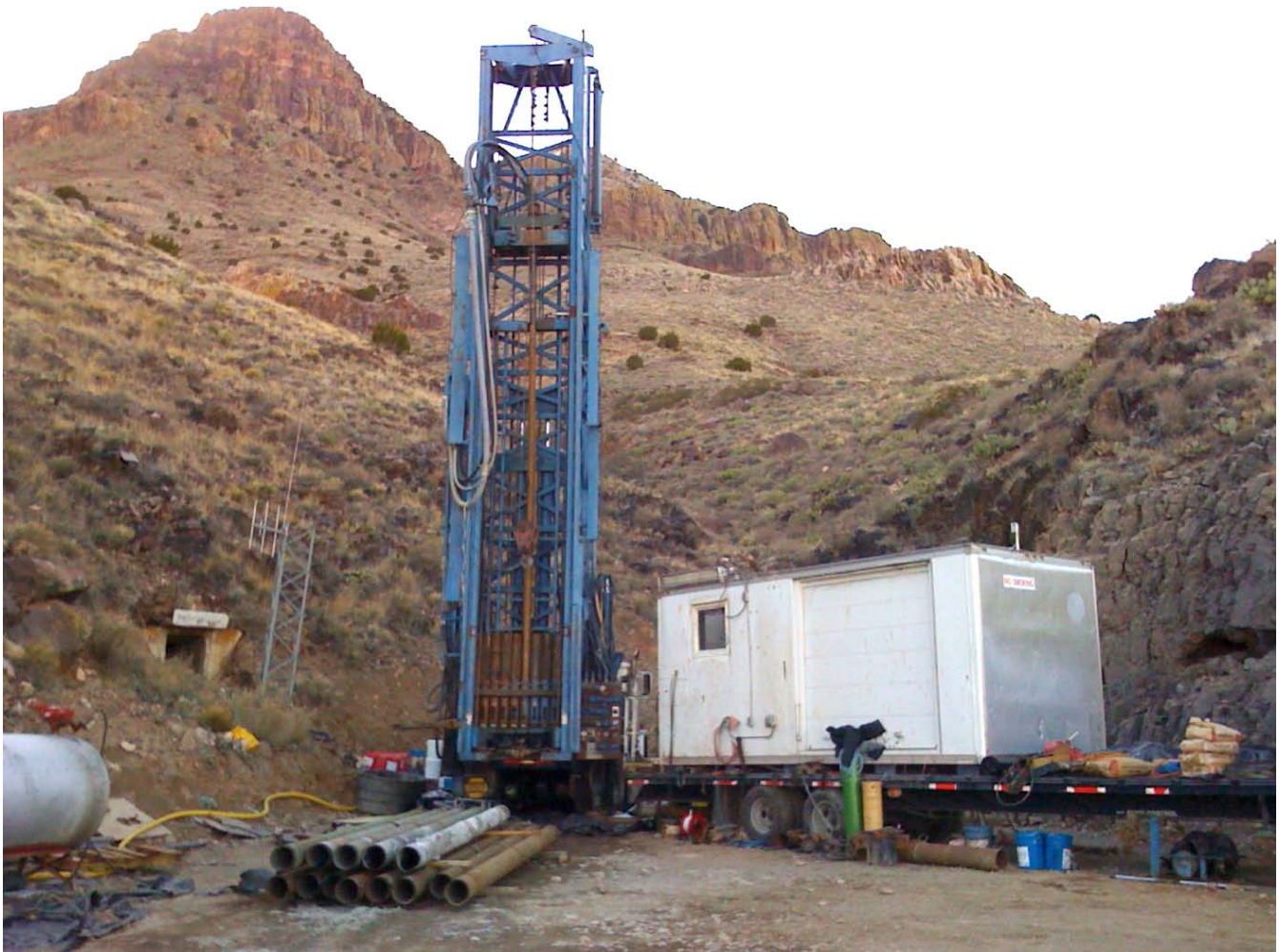
Drilling rig used in the slim hole drilling operation.
