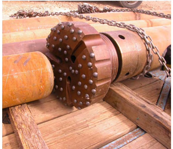
Drill bit used in the slim hole drilling operation.
