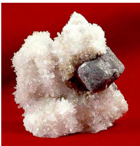
A rounded galena crystal from the Hansonburg mining district, Socorro County, New Mexico. This crystal contains almost no silver. This specimen is typical of a sedimentary lead deposit. Photo courtesy of Debra Wilson, New Mexico Bureau of Geology museum specimen #11454.
