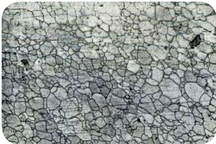
A microscopic image of a metamorphosed galena sample magnified 100x. A standard optical microscope is limited in the amount of magnification it can produce because of lens distortion. A lens bends light, and more bending (higher magnification) results in more distortion and diffraction (separation of light), especially on the edges of the lens. With high magnification, you must look through the middle for the best image. Image modified from Ramdohr 1969, The ore minerals and their intergrowths , 3rd ed., Pergamon Press, New York, 1,174 pp.
