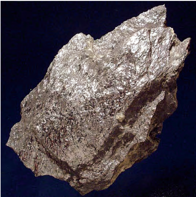
Sparkly, “steely” silver galena contains significant silver, as in this deformed galena schist from the Pecos mine, San Miguel County, New Mexico. Photo courtesy of Virgil W. Lueth, museum specimen #12444.
