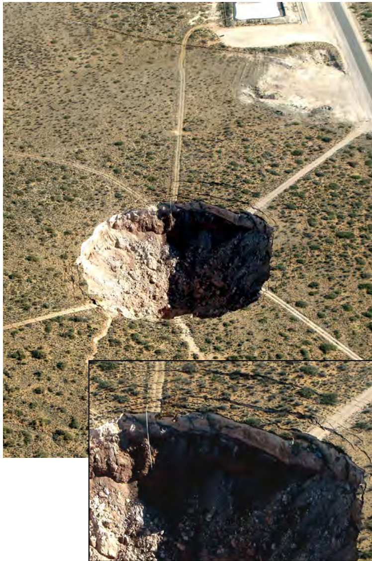
The JWS Sinkhole in Eddy County, New Mexico is over 300 feet across. The inset is a close-up view of ring fractures formed around the edge of the sinkhole. Photo courtesy of Lewis Land, National Cave and Karst Research Institute.
