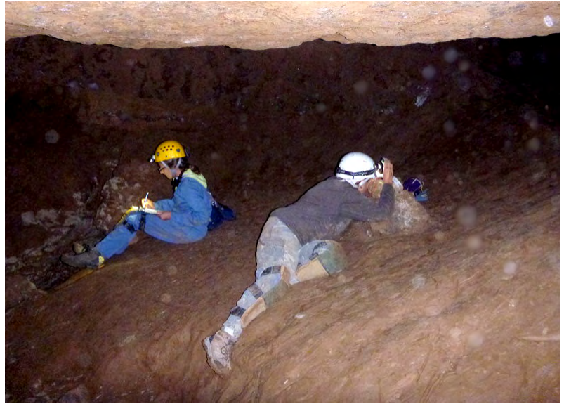
Surveying a passage in Fort Stanton Cave, New Mexico. The sketcher (Janice Tucker) is recording data while Linda Starr is measuring inclination (the vertical angle between two survey points). Photo courtesy of the Fort Stanton Cave Study Project and Jennifer Foote.
