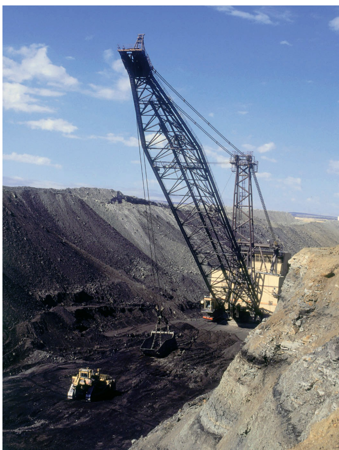
This dragline is mining coal at the Lee Ranch Mine, McKinley County, New Mexico. Photo courtesy of Peabody Energy.
