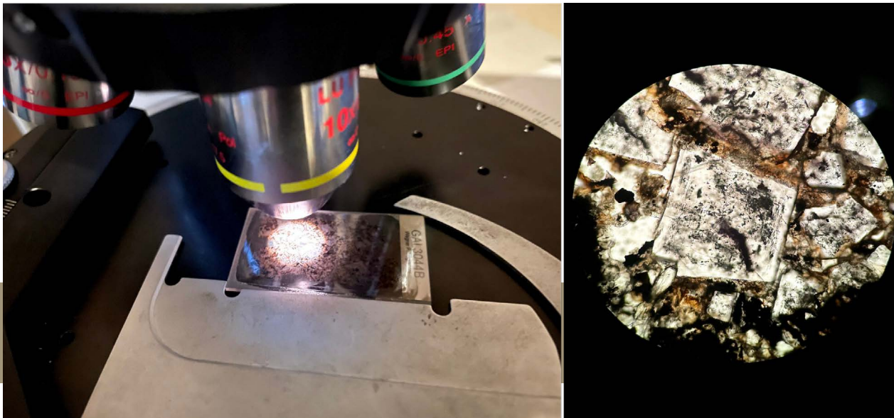
Figure 2. At left, a thin section under the microscope in NMBGMR's Ore Deposits and Critical Minerals Lab. At right, a transmitted light view shows a cross section of cubic fluorite crystals. Photos by Alex Gysi
