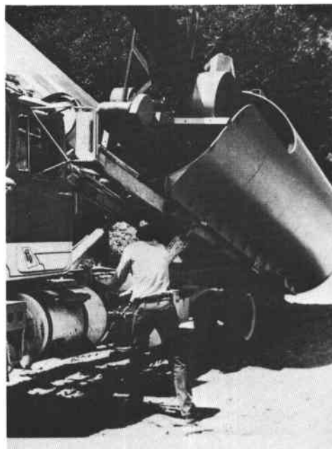
FIGURE 6—UNIT IS DRAWN UP ON BED JUST BEYOND CENTER OF GRAVITY. Courtesy Challenge Mining Company.
