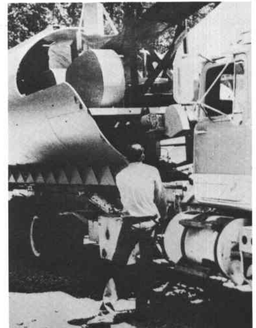
FIGURE 7—BED IS LOWERED, UNIT ROLLED FORWARD AND LOCKED INTO PLACE. Courtesy Challenge Mining Company.
