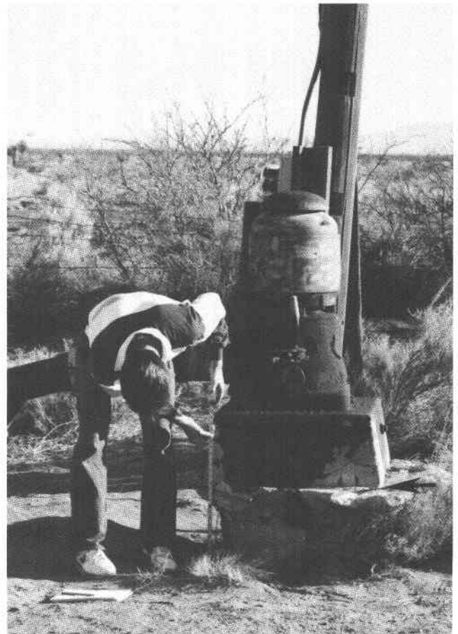
FIGURE 8—Photograph showing protruding water well A. Original land surface is indicated by arrow. Photograph was taken in April 1988.
