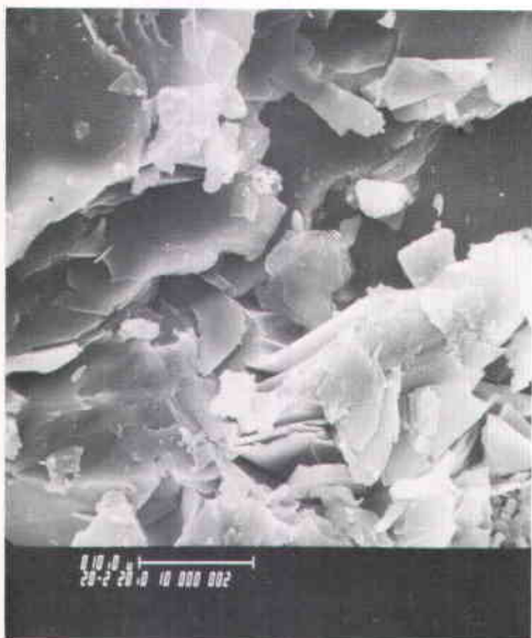
FIGURE 3—SCANNING ELECTRON MICROSCOPE PHOTOMICROGRAPH OF TALC PARTICLES; enlargement approximately \times 1,400 (courtesy University of New Mexico School of Medicine, by D. G. Brookins and R. Hicks).
