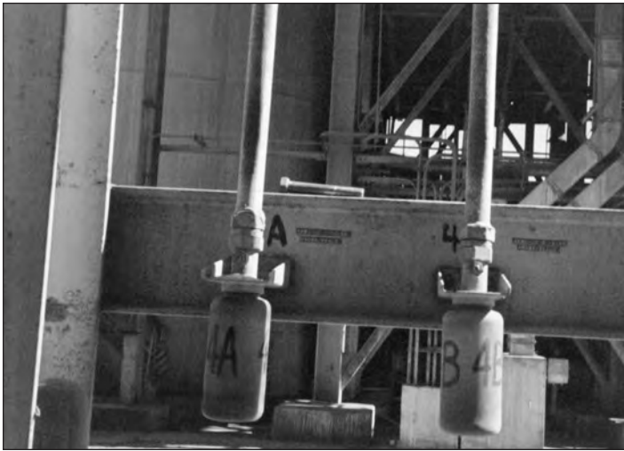
FIGURE 9—Phoenix Cement sampling vials for each generating unit at Cholla Generating Station. Ash samples are collected every 2 hrs for analyses.
