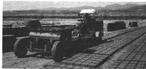
FIGURE 3—SELF-PROPELLED MECHANICAL ADOBE LAYER LOCATED AT THE ADOBE YARD IN SAN JUAN PUEBLO, NEW MEXICO.
