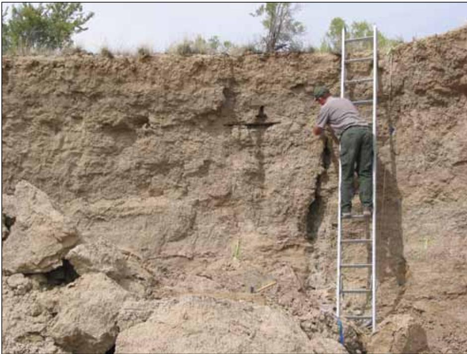
FIGURE 11—L30 stratigraphic section measured in September 2005. Pale-green surveyor tape marks detrital charcoal. Blue tape marks depth in meters. The Appendix gives details of measured sections.
