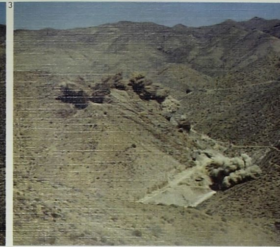
THE BLAST—BEFORE, DURING AND AFTER Fifty-pound bags of explosives are loaded into tunnels in the Old Reliable deposit (1), then detonated by primacord (2), in a record-setting blast (3, 4, 5) which crushed ore in the deposit, but left the surface above it largely intact (6).
