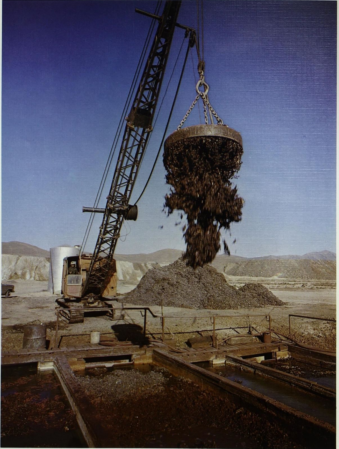
Crane-mounted electromagnet drops iron into precipitation cells at Big Mike
