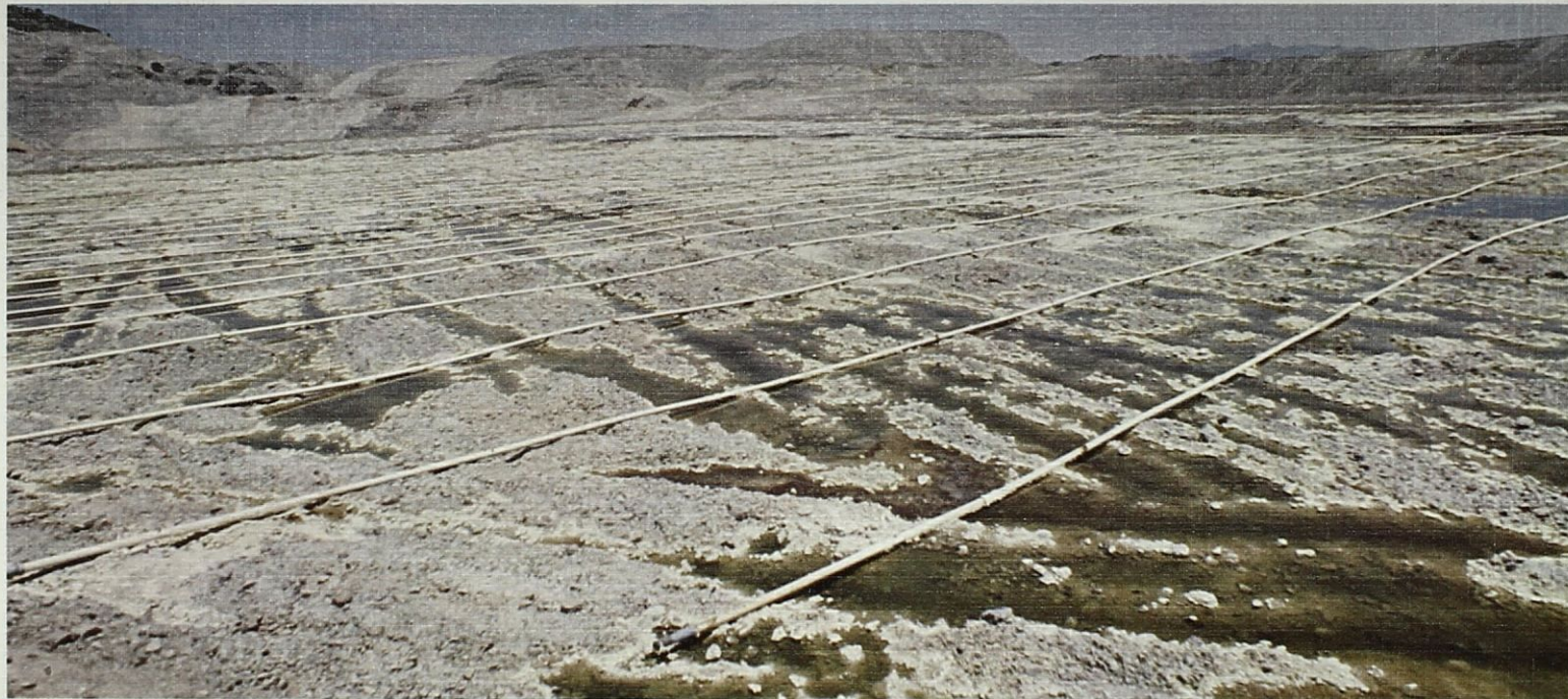
Leaching Copper Ore at the Bluebird Mine
