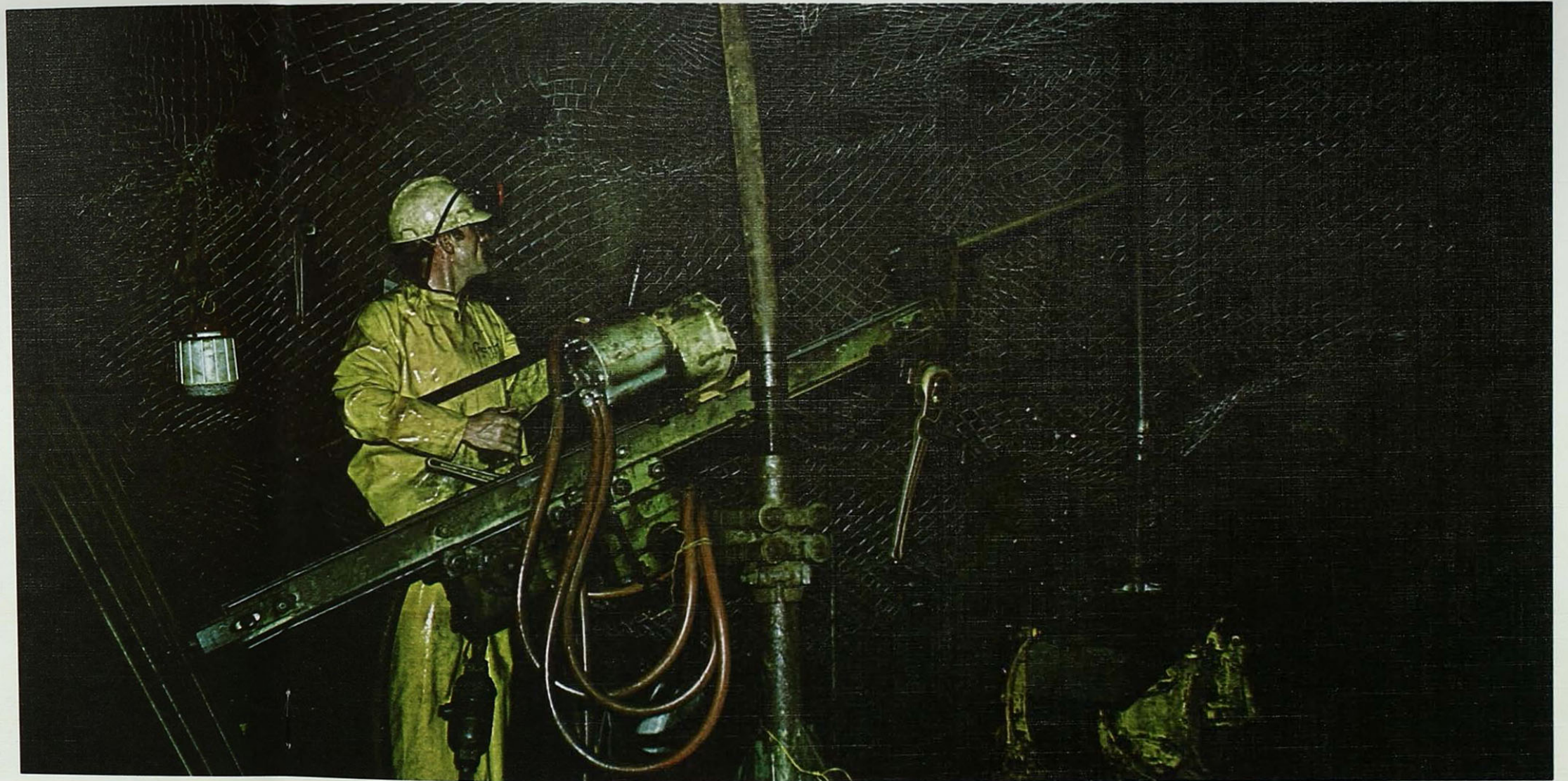
Long Hole Drilling at the Johnny M
