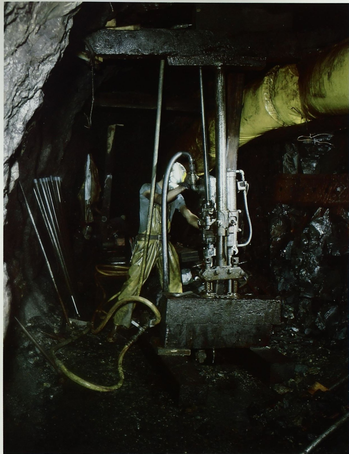
Core Drilling Underground at the Revenue-Virginius Mine
