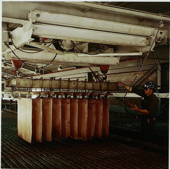
Copper cathodes from the world's first solvent extraction-electrowinning plant.
