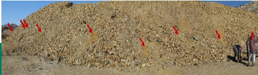
Eroded oxidation profile in a rock pile at Copper Flat
