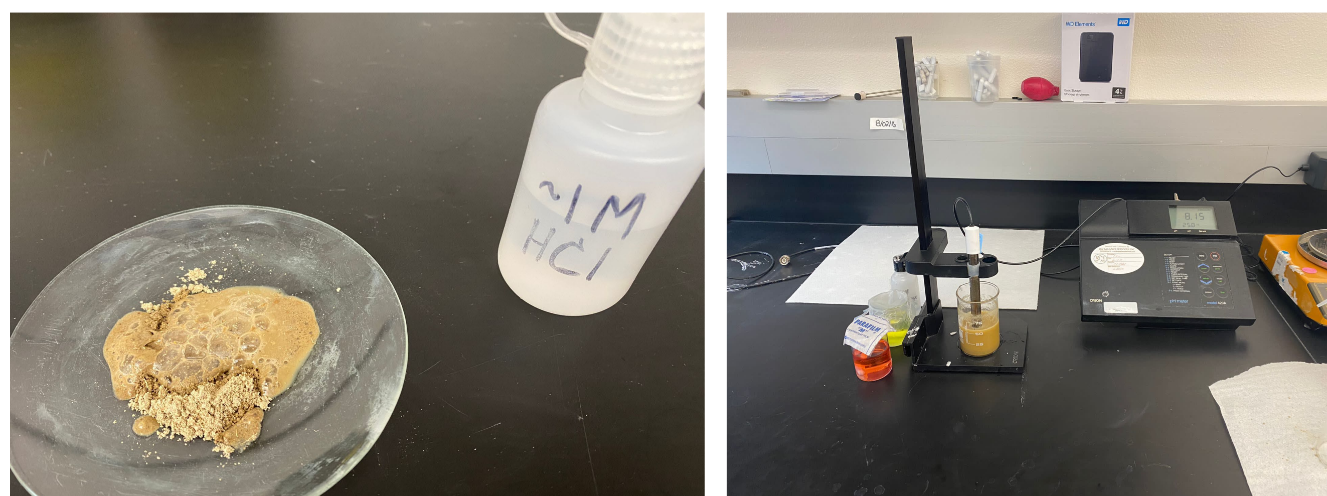
FIGURE 6: Laboratory test on sieved samples, Fizz test(left) and Paste pH test (right)
