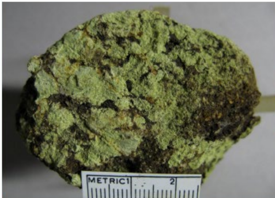
Supergene Monazite replacing massive apatite mineralization Araxá, Brazil Furo O-IXMO, 191.25 meters (12-A-1)
