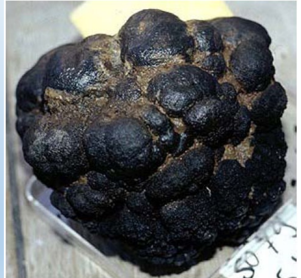
Figure 1. A cluster of manganese nodules 20 cm in diameter and weighing 25 kg. Photograph courtesy of the German Federal Institute for Geosciences and Natural Resources (BGR).
