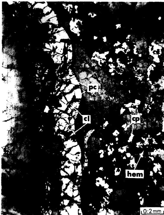
Fig. 11. A pitchblende vein (*pc*), accompanied by chlorite (*cl*); (*cp*) = chalcopyrite, (*hem*) = hematite. RAH occurrence, Great Bear Lake area, Northwest Territories, Canada. Photomicrograph, reflected plain light.
