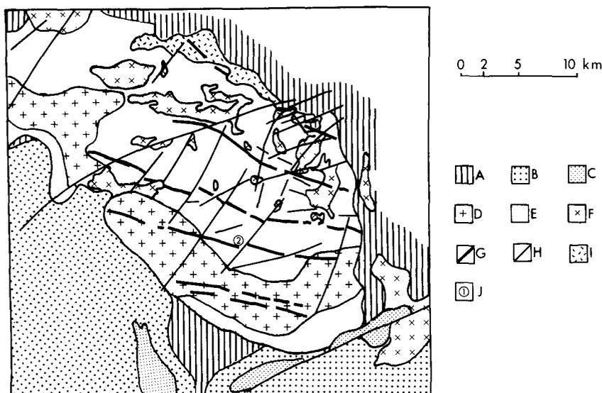
Fig. 4. Location of intragranitic uranium vein deposits in Xiazhuang area, Guangdong Province, China. *A*=Early Paleozoic rocks; *B*=Devonian rocks; *C*=Late Cretaceous red beds; *D*=coarse-grained biotite granite; *E*=medium- to fine-grained biotite granite; *F*=two-mica granite; *G*=intermediate to mafic dyke; *H*=quartz vein and silicified zone; *I*=dacite; *J*=uranium deposit; (1)=Zhushanxia and (2)=Shijiaowei. After Li Tiangang and Huang Zhizhang (1986).
