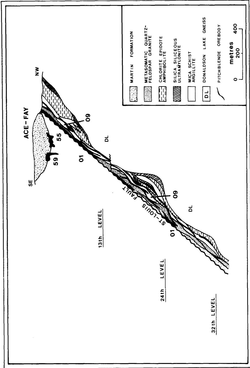
Fig. 13. Vertical cross-section through the Ace-Fay ore bodies, Beaverlodge area, Saskatchewan, Canada. Modified from Eldorado mine documentation.
